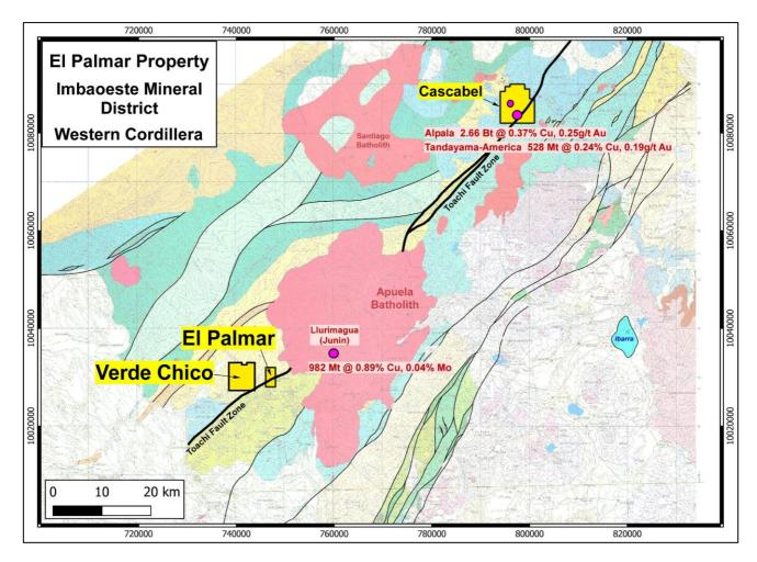
**Figure 3:** Location of the El Palmar project relative to the giant Llurimagua, Alpala- and Tandayama-America (Cascabel) porphyry deposits, and the Toachi fault system.
