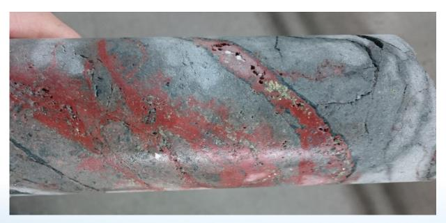
Figure 3 - Drill core from NDD 001 at 81m showing albite alteration and pyrite-chalcopyrite in veins
