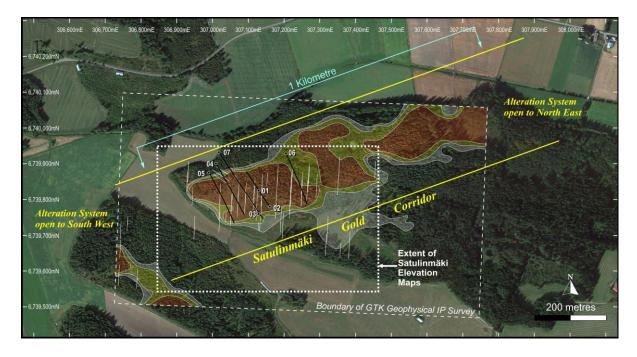
Figure 5: Plan view of Satulinmaki Prospect showing extent of drilling, existing IP survey, structural corridor and extent of Satulinmaki Elevation Maps.
