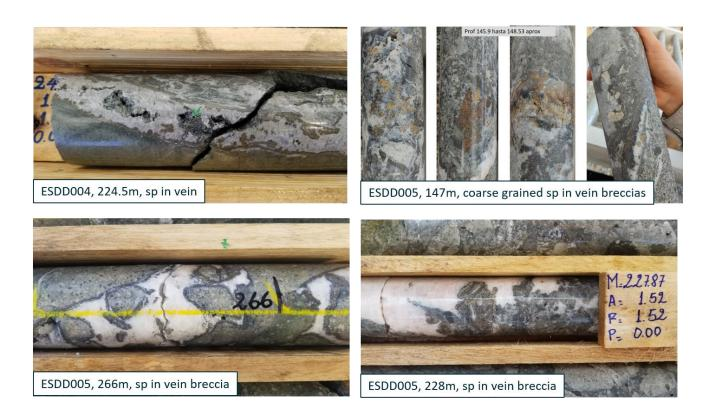
**Figure 1:** Photographs of drill core from drill holes ESDD004 and ESDD005 showing calcite veining and vein breccias with sphalerite (sp)
