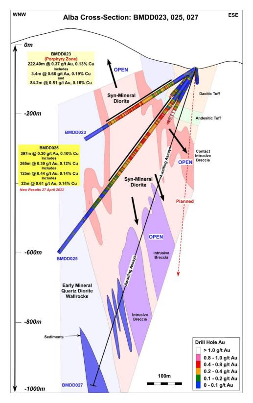
**Figure 3:** Alba cross section showing holes BMDD023, 23 and 27. This section is located up to 100m to the south of the section in Figure 2.
