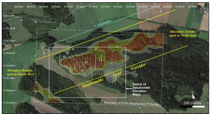
**Figure 3:** Plan view of Satulinmaki Prospect showing extent of drilling, existing IP survey, structural corridor and figures 1 & 2 as extent of Satulinmaki Elevation Maps.
