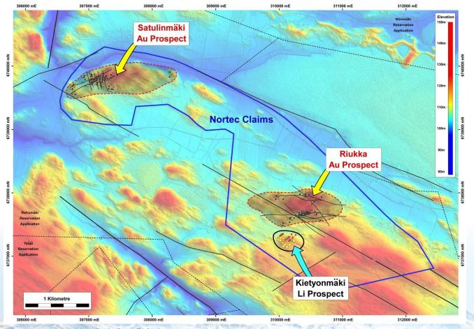
Figure 4: location of Satulinmäki and Riukka showing small areas tested by drilling to date.
