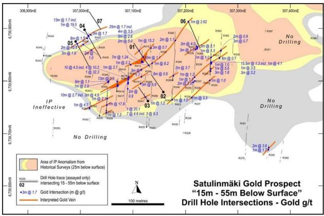
Figure 1: Plan map of assay results from Avalon and GTK drilling at 15m to 55m below surface
