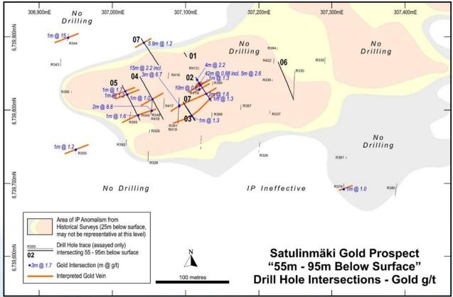
**Figure 2:** Plan map of assay results from Avalon and GTK drilling at 55m to 95m below surface. The area of IP anomalism is shown at 25m below surface and was ineffective below this depth.
