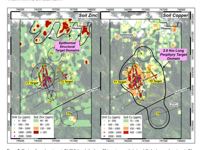
**Figure 7:** Cluster of porphyry targets T1 (El Palmar), the large T2 target currently being drilled, plus porphyry targets T4 and T5. To date T1, T2, and T5 are mineralised. Epithermal target areas in the north, of which only Tituana has been drilled to date.
