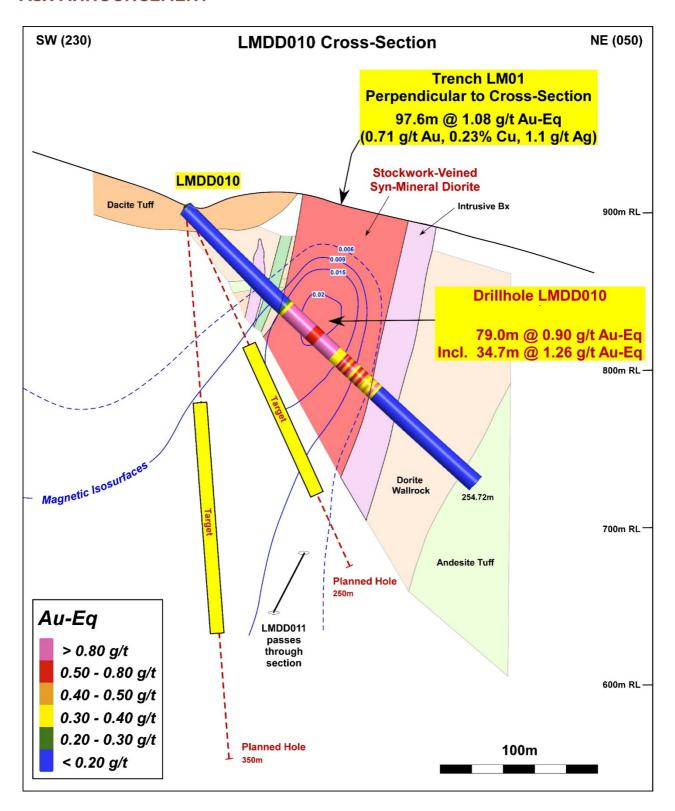
**Figure 5:** LMDD010 cross section showing surface trench and other nearby drill holes and interpreted target zone based on geological and geophysical (magnetics) interpretation.
