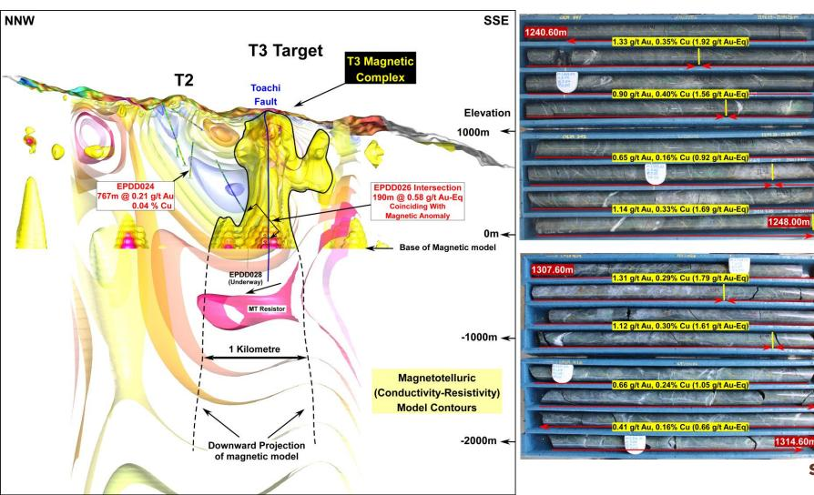
EPDD026 grades suggest the T3 system can deliver very high grades relative to other porphyry deposits
