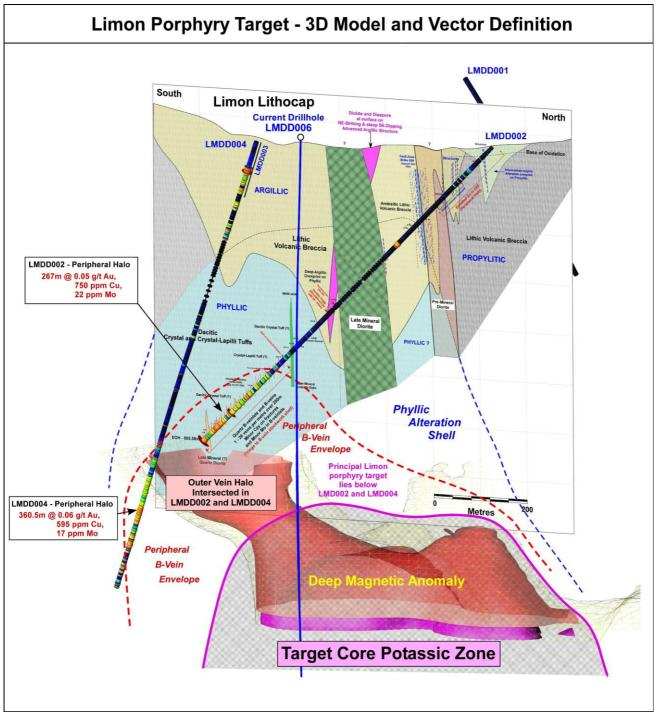
Figure 6: Limon Porphyry target showing oblique view (slightly inclined towards the WSW) of holes LMDD002 and 004, and current hole LMDD006. Multiple datasets are supporting a target below and between holes 002 and 004, with the extensive low-grade Cu-Au-Mo intersections in LMDD002 and LMDD004 coming from the outer-most vein halo.
