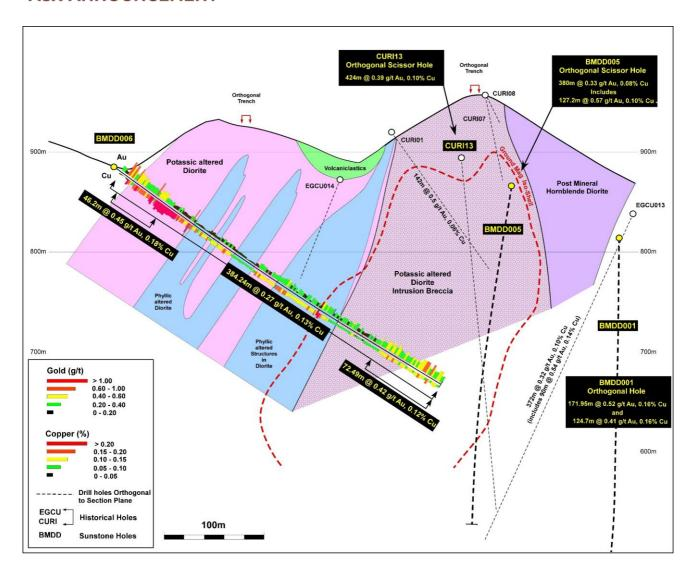
Figure 4: Cross section on trace of hole BMDD006, and showing the trace of BMDD005 some of which is on section
