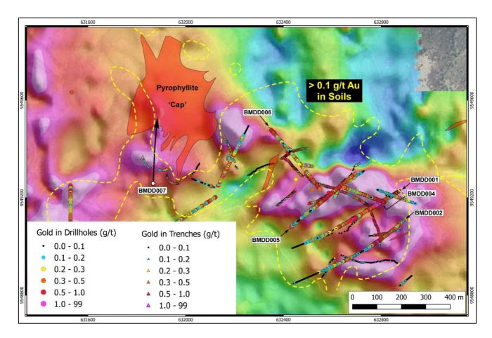
Figure 3: Plan view and drill status plan of the Bramaderos Main porphyry target showing recently processed ground magnetic data as Reduced-to-Pole (RTP) imagery. The anomaly shape in the area of drilling BMDD001 – 007 has been refined from the original interpretation of the heli-magnetics data and is currently undergoing detailed review.
