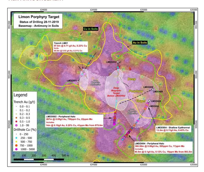
Figure 5: Limon Porphyry target showing drill status over compilation geology and surface geochemistry. Current diamond drill hole LMDD006 is shown as the black dashed line, and will test a target underneath hole LMDD002, and between holes LMDD002 and LMDD004. The target is defined on the basis of geology, 3-D modelling of detailed ground magnetics, and geochemistry.
