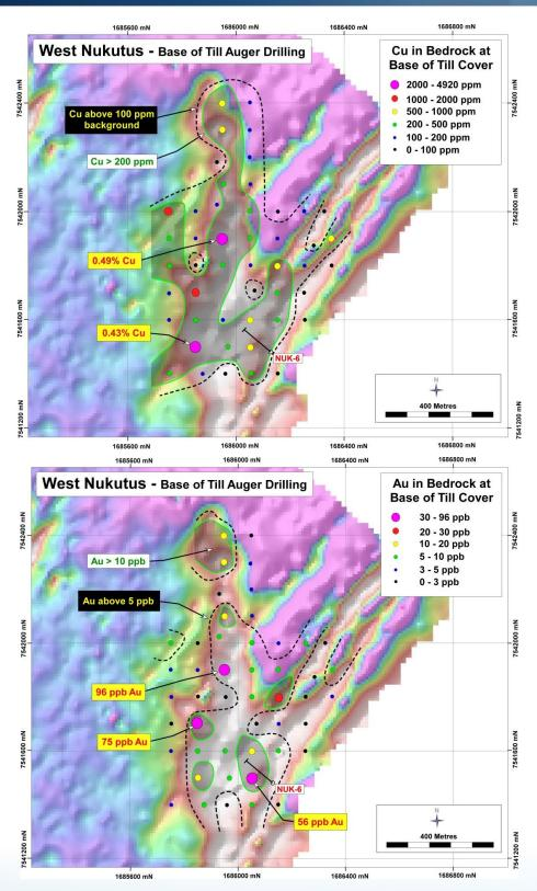
Figures 3a (top) and 3b (bottom): West Nukutus target – images showing TMI magnetics, auger holes drilled on a 100m by 100m grid and historic hole NUK 6.Copper anomalism (top) plus gold anomalism (bottom).
