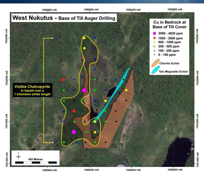
Figure 2: West Nukutus target – showing auger holes drilled on a 100m by 100m grid, and copper assay values in ppm plus an outline of visible chalcopyrite mineralisation at the top of the basement rocks and just below the transported till cover rocks.
