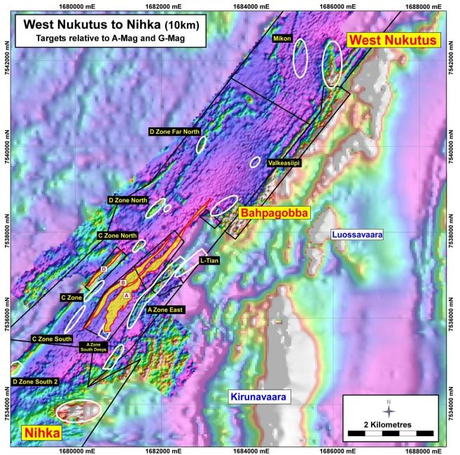
Figure 1 – Location of the West Nukutus target relative to the Viscaria Copper Project copper deposits (A, B & D Zones). Background image is TMI ground and airborne magnetics
