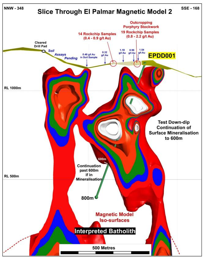
**Figure 6:** Slice through the 3-D model of the El Palmar magnetic target showing the location of the planned hole EPDD001 and showing surface rock chip and soil gold results. EPDD001 will drill below mineralised stockwork shown in Figure 3.
