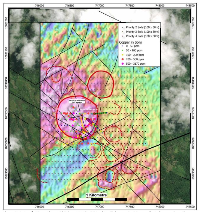
**Figure 4:** Status of soil sampling at El Palmar. Priority 2, 3 and 4 soils have not yet been collected so are shown here as planned sample points only. The soils over the main El Palmar magnetic anomaly are showing coincident anomalous copper and gold.
