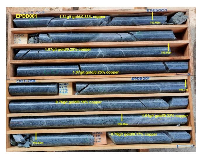
**Figure 5**: Photograph of drill core from EPDD001 from 152.5m to 159.5m showing sampling intervals and gold and copper assay results.
