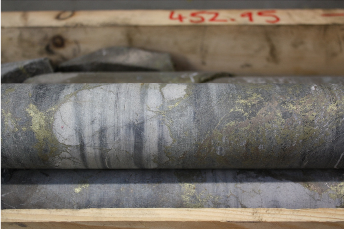
Figure 4 - Typical Copper Mineralisation Intersected in Drill Hole VDD0125
