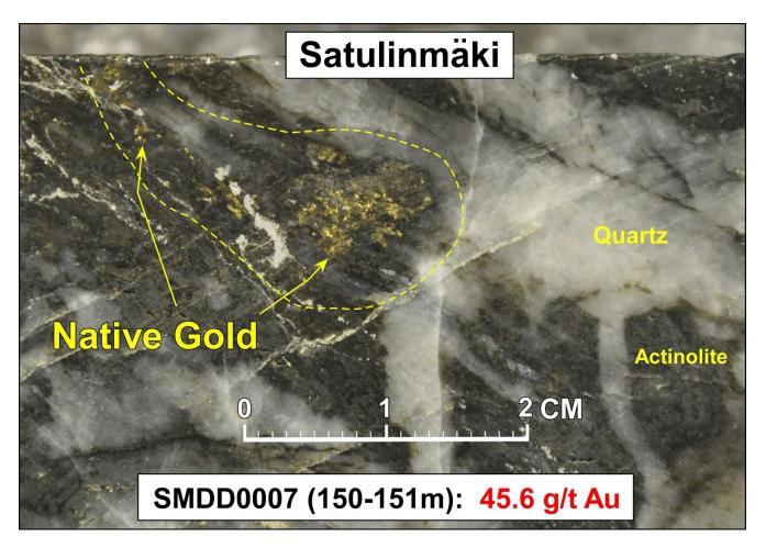
Figure 2: Visible gold in hole SMDD007 at 150m
