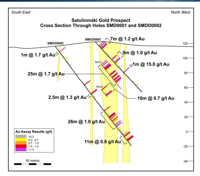
Figure 4: Cross section through drill holes SMDD001 and 002 at Satulinmäki gold prospect.
