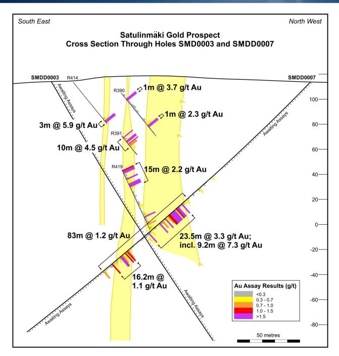
Figure 3: Cross section through drill holes SMDD003 and 007 at Satulinmäki gold prospect.
