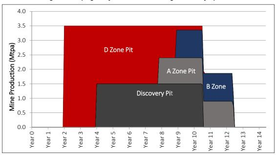
Figure 3: Scoping Study Mine Production Target Profile by Open Pit
