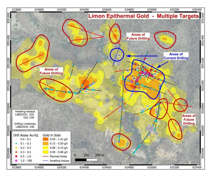
**Figure 3:** Limon gold in soils map showing extensive anomalous gold over an area of 1.7km x 700m. The blue circled areas are where current drilling is active. Red circled areas show the multiple epithermal gold-silver targets. Several of these demonstrate direct evidence of epithermal mineralisation based on historical drilling.
