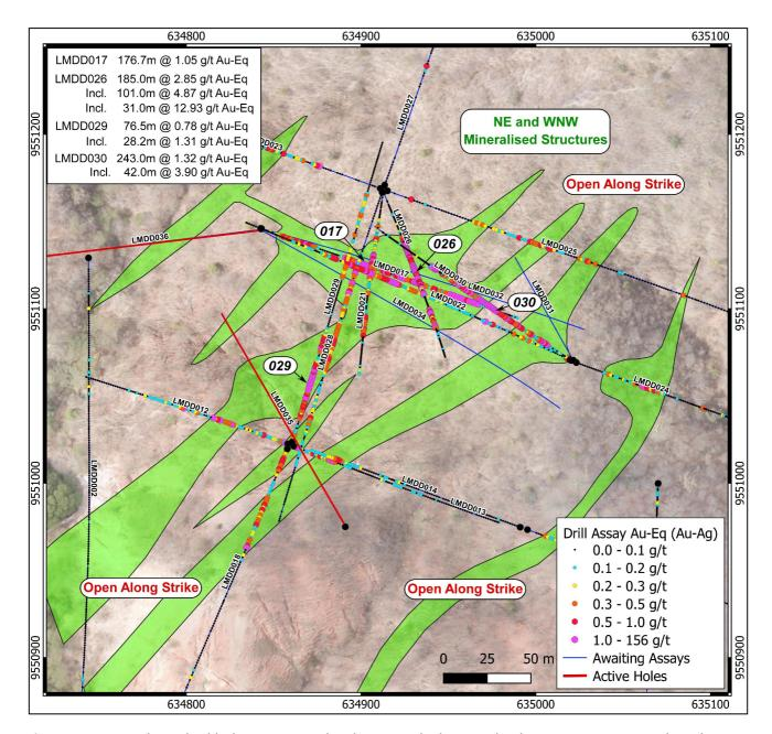
**Figure 1:** Limon epithermal gold-silver system in plan showing multiple mineralised structures in green. High grade domains are at intersections of NE and WNW trending structures. Several additional targets have been defined based on gold-in soil and zinc-in-soil anomalies, and structural interpretation. See Figures 2 and 4 for sections through this system, and Figure 3 for a broader context within the very large Limon target area.
