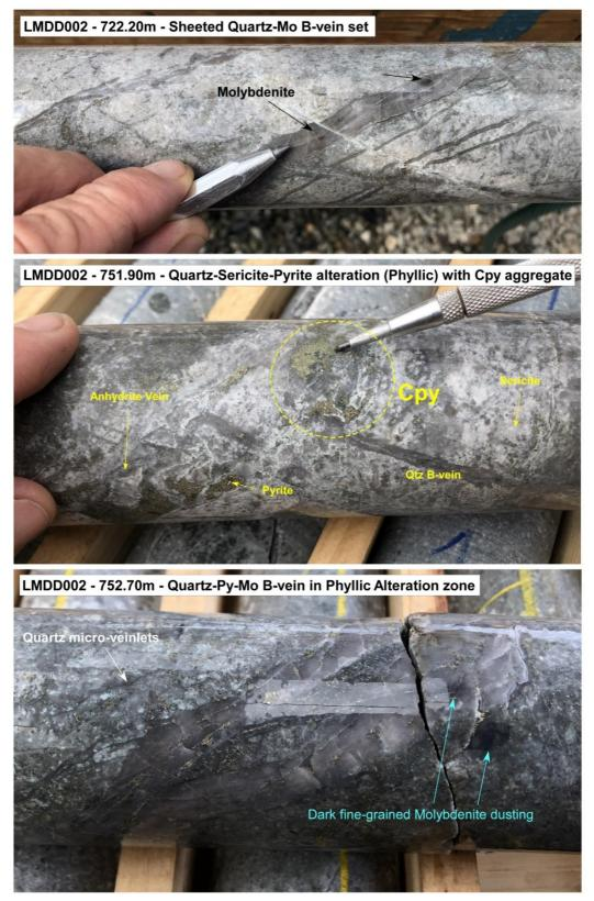
Plates 2-4 – Variety of porphyry B-vein textures seen in LMDD002 (Cpy = chalcopyrite).
