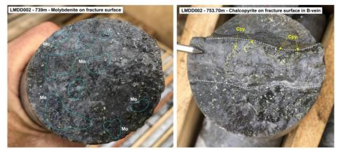
Plates 6 and 7– Molybdenite and chalcopyrite smears and disseminations on some fracture surfaces in LMDD002.
