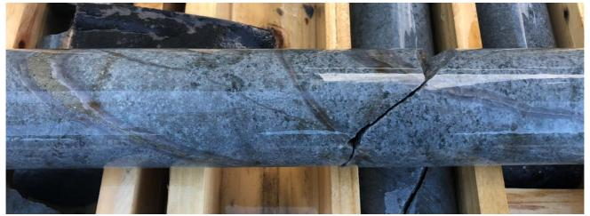
*Plate 1 – Development of B-generation quartz + sulphide veins at Limon in Hole LMDD002 (705.4m depth) in intensely phyllic-altered intrusive.*
