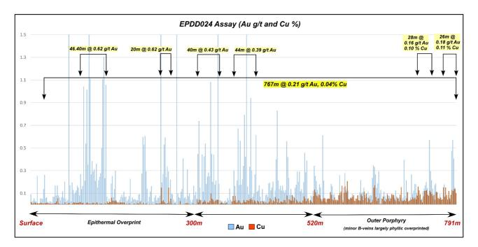
**Figure 4:** Drill hole EPDD024 down hole assay plot clearly showing upper-level epithermal overprint dominated by gold, and lower copper-gold porphyry signature.
