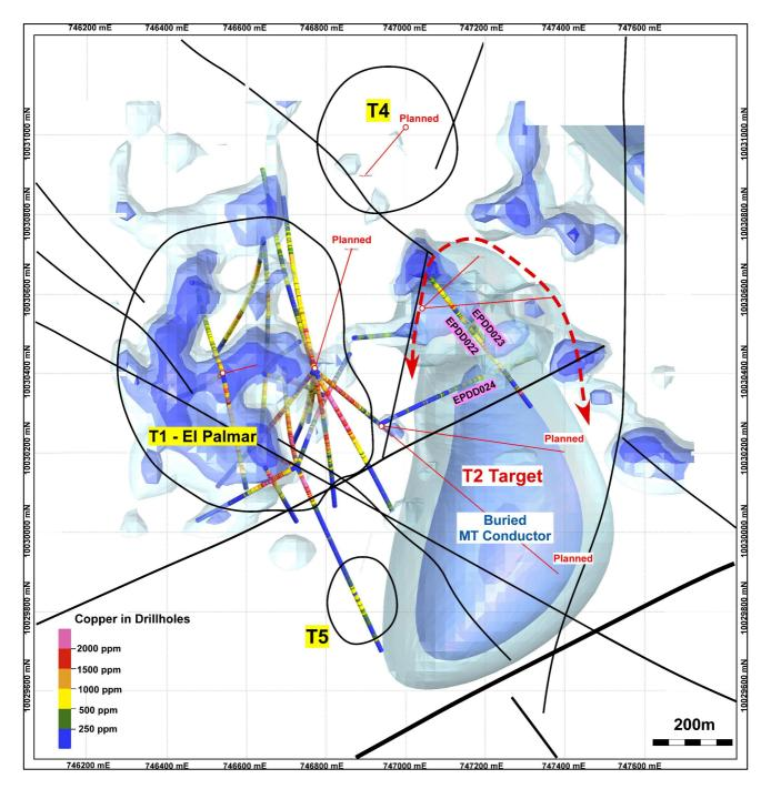
Figure 2: Close up porphyry targets T1 (El Palmar) and large T2 target plus porphyry targets T4 and T5.
