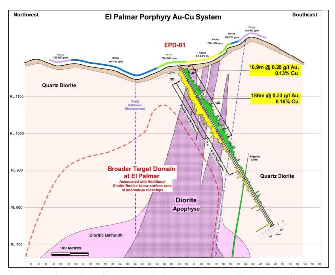
**Figure 9:** Section diagram showing the target zone at El Palmar as currently interpreted from surface sampling and one drill hole on section. 3-D magnetic modelling will refine this target definition to be drilled.
