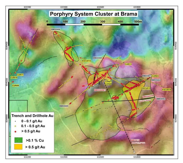
**Figure 4:** Same image as Figure 2 showing the RTP magnetics as a backdrop and the circular magnetic response that is attributed to an outer and shallow mineralised intrusive breccia, and an inner and vertically extensive stockwork porphyry domain.
