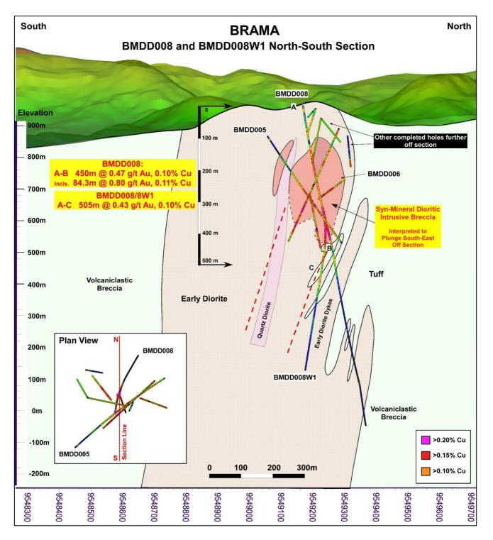
Figure 1: Brama cross section showing drill holes BMDD008 and new wedge hole BMDD008W1.
