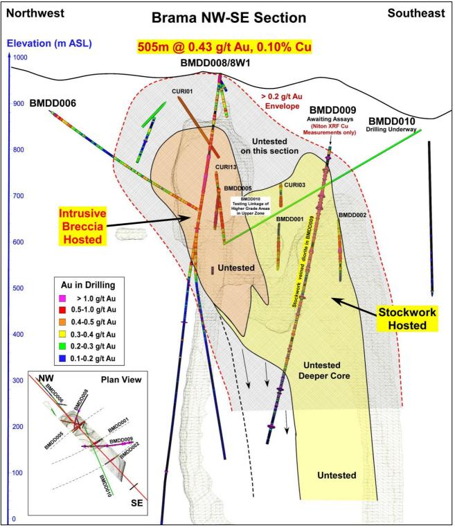
**Figure 2:** Brama cross section showing geological model and relationship between stockwork veined diorite mineralisation and intrusive breccia hosted mineralisation.
