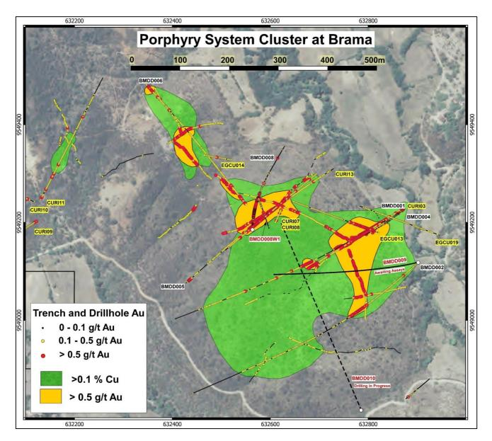
**Figure 3:** Brama gold-copper porphyry plan view showing higher grade gold domains within a broad lower grade copper halo covering 700m x 500m. Also showing locations and results for holes BMDD008 and W1, and locations for holes 9 and 10
