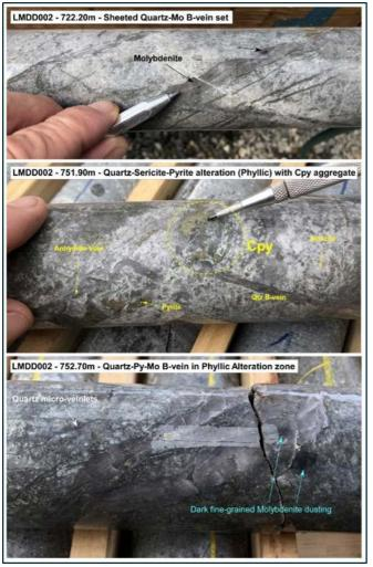
Figure 4: Variety of porphyry B-vein textures seen in LMDD002 (Cpy = chalcopyrite).
