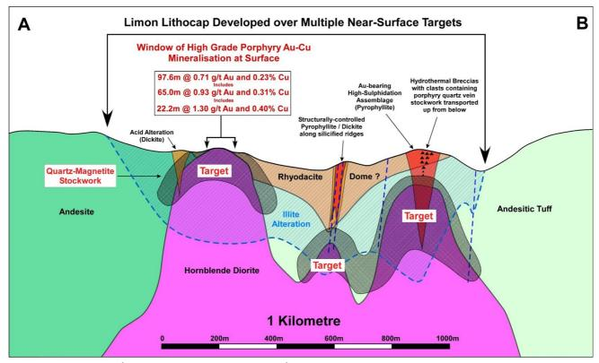
Figure 2: Long-section (oriented WNW-ESE; see Figure 1) through the Limon porphyry Au-Cu prospect, illustrating key geological features that suggest an extensive underlying mineralised porphyry gold-copper system below the leached clay-altered lithocap (illite). Strongly mineralised diorite outcrops as a window through an overlying and altered rhyodacite body.
