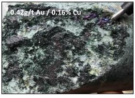
**EPDD001 320m.**Coarse-grained bornite along shear zone + actinolite.
