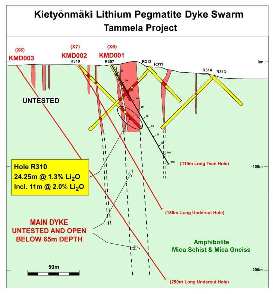
Diagram showing a section through the Kietyönmäki deposit on the traverse of KMD001.
