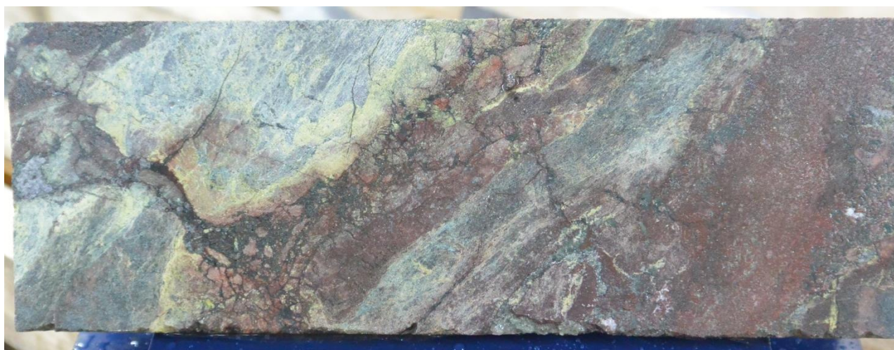
Figure 3: NDD 001 at 37.75m down hole, showing altered and brecciated host rocks with magnetite and hematite alteration.
