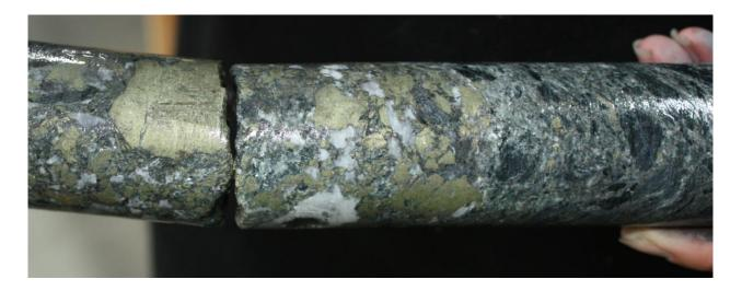
Figure 4: VDD 186 drill core at 536.2m showing breccia texture with significant chalcopyrite.
