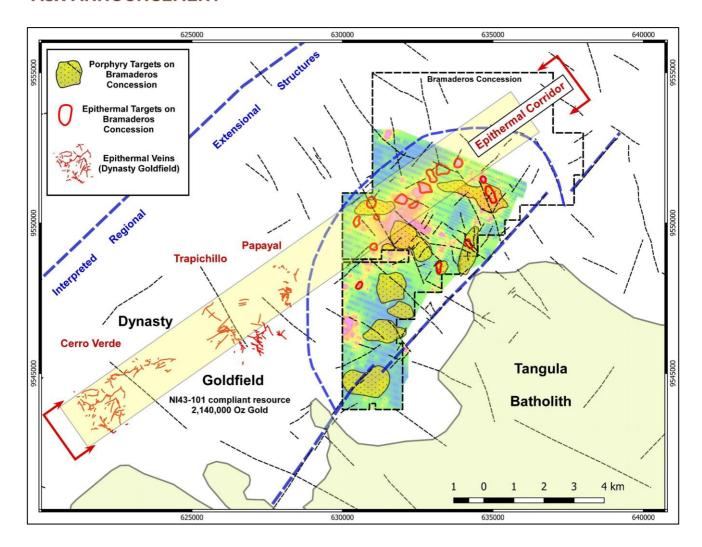
Figure 4: The Bramaderos concession showing the multiple porphyry gold-copper systems and the extension of the 2 million ounce Dynasty Goldfield epithermal belt.
