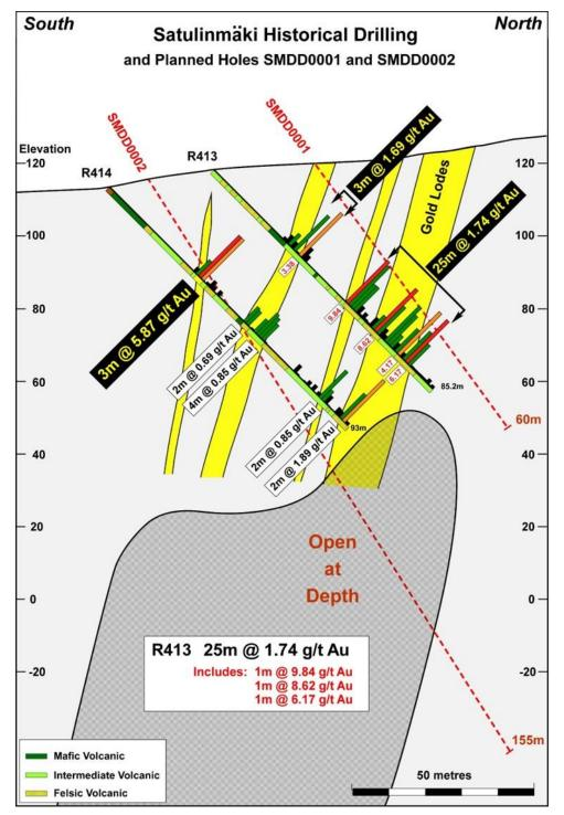
Figure 3: Cross section showing target zone down plunge from mineralised horizons in historical holes R413 and R414.
