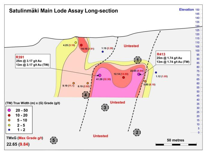
Figure 4: Long section on the main gold bearing zone showing existing shallow historical intersections, and pierce points of the proposed drill holes 1 to 5. The 5 proposed drill holes have also been planned to intersect several sub-parallel gold horizons parallel to this main zone.
