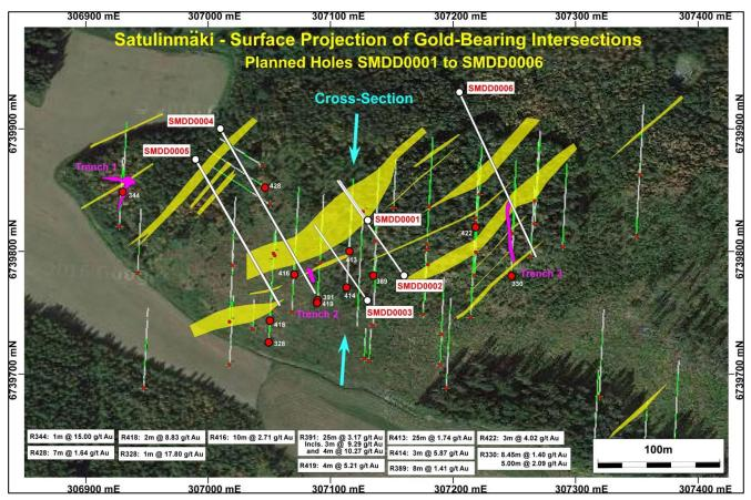
Figure 2: Satulinmäki gold prospect showing interpreted NE trending gold bearing vein systems. Figure 3 cross section is shown through the main target vein. Collar positions of historical holes with red dots and grey, green traces. Proposed holes SMD001 to SMD006 are shown in white.
