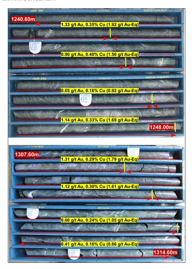
**Figure 10:** Drill core from EPDD026 over the interval 1240 – 1314m showing strong stockwork veining and high grade gold and copper assays.
