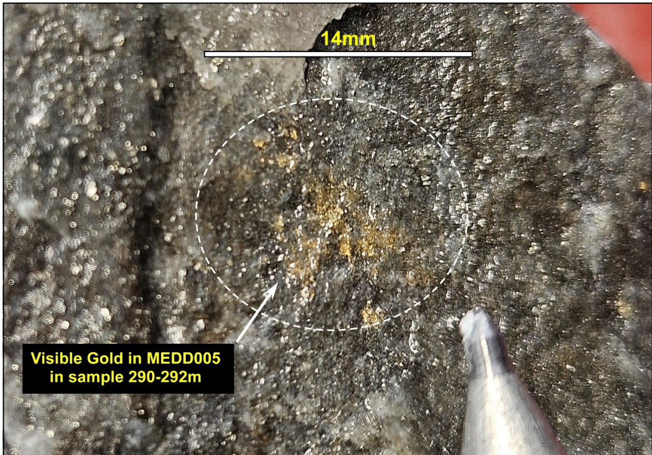
Image 2: Native gold observed along a fracture near the bottom of MEDD005 between 290m and 292m downhole. The broader interval, containing the other half core to this sample, assayed 9.35m @ 17.23 g/t Au-Eq 7 . The gold occurs as fine disseminations along a fracture surface that cuts volcanosedimentary wallrocks to the Melonal porphyry system. Minerals in this interval include native gold (trace quantities <0.01%), chlorite (~10%), anhydrite (~4%) and local andradite garnet (~2%). The remaining mineralogy comprises quartz (~15%) and feldspar (~50%) in siliciclastic, volcanic-derived, finely-bedded tuffaceous sediments. A 20m interval near the bottom of MEDD005 has been re-sampled for repeat assay. Visual estimates of mineral abundance should never be considered a proxy or substitute for laboratory analyses where concentrations or grades are the factor of principal economic interest. Visual estimates also potentially provide no information regarding impurities or deleterious physical properties relevant to valuations.
