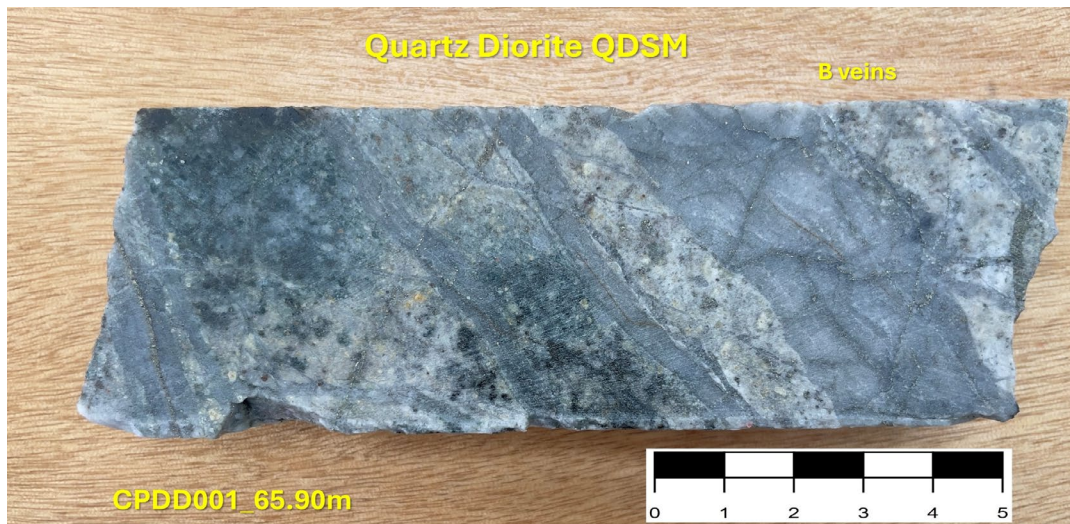
Figure 3: Photo of representative drill core from CPDD001 at 65.90m (0.55 g/t Au-Eq 2 ); in assay 0.46 g/t Au, 0.06% Cu in porphyry-veined syn-mineral diorite. Location at P1 in Figure 2. This sample shows vein-hosted mineralisation in a quartz-diorite host rock, with vein density around 25 veins (>1cm wide) per metre. Mineralisation comprises disseminated chalcopyrite within the veins and in the wallrock (<0.2% chalcopyrite) in association with magnetite (3%), chlorite (6%) and sericite (25%).
