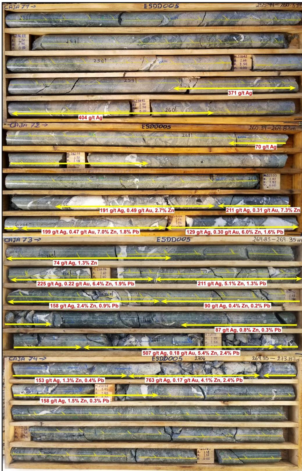
**Figure 2:** Drill core photograph from ESDD005 showing wide intervals of veined and brecciated rock containing very significant assays of silver, zinc, lead and gold. The interval shown is 259.1m to 270.7m, 11.6m at 167.4g/t silver, 0.16g/t gold, 0.8% lead and 2.1% zinc, with locally very high grade silver up to 404g/t.
