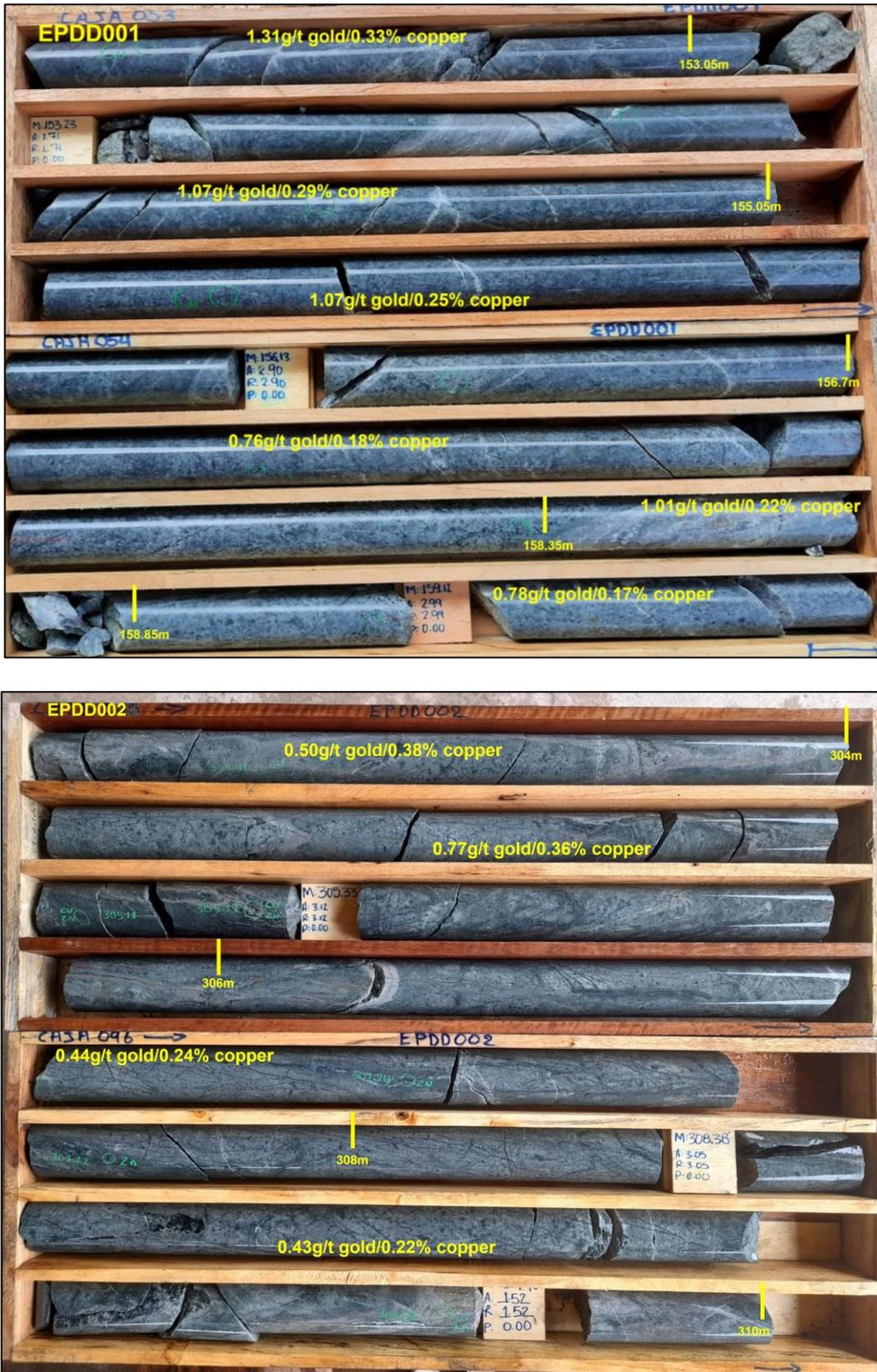
Figure 3: Photograph of drill core from EPDD001 from 152.5m to 159.5m, and EPDD002 from 303m to 310m showing sampling intervals and gold and copper assay results.
