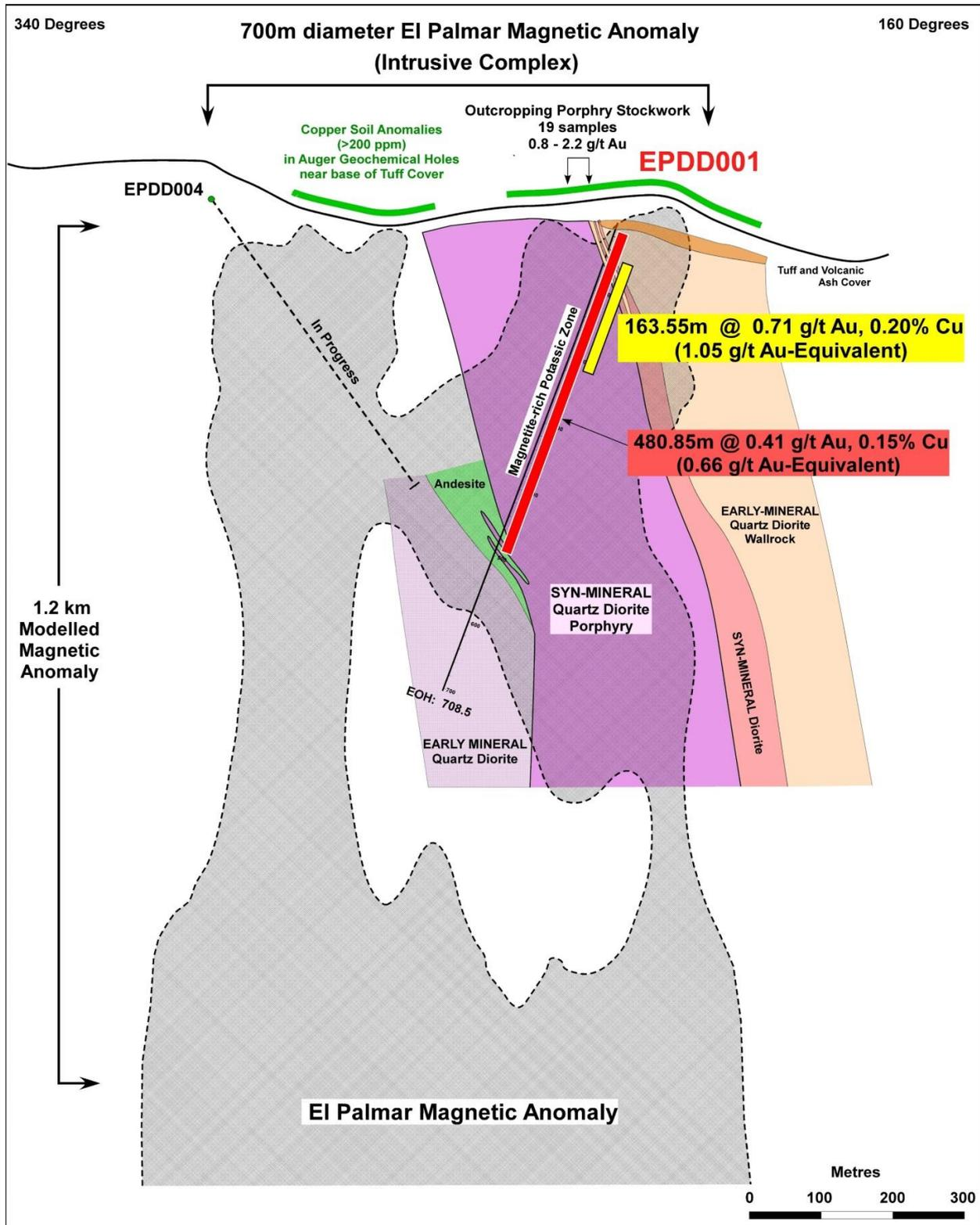
**Figure 2:** Cross section through EPDD001 at El Palmar. The 480.85m long intersection of porphyry gold and copper mineralisation is hosted by a quartz diorite porphyry intrusion that coincides with the southeast section of a 700m diameter magnetic intrusive complex. Surface copper and gold responses in auger soil samples (Figure 4) suggest significant portions of this magnetic complex may be mineralised.
