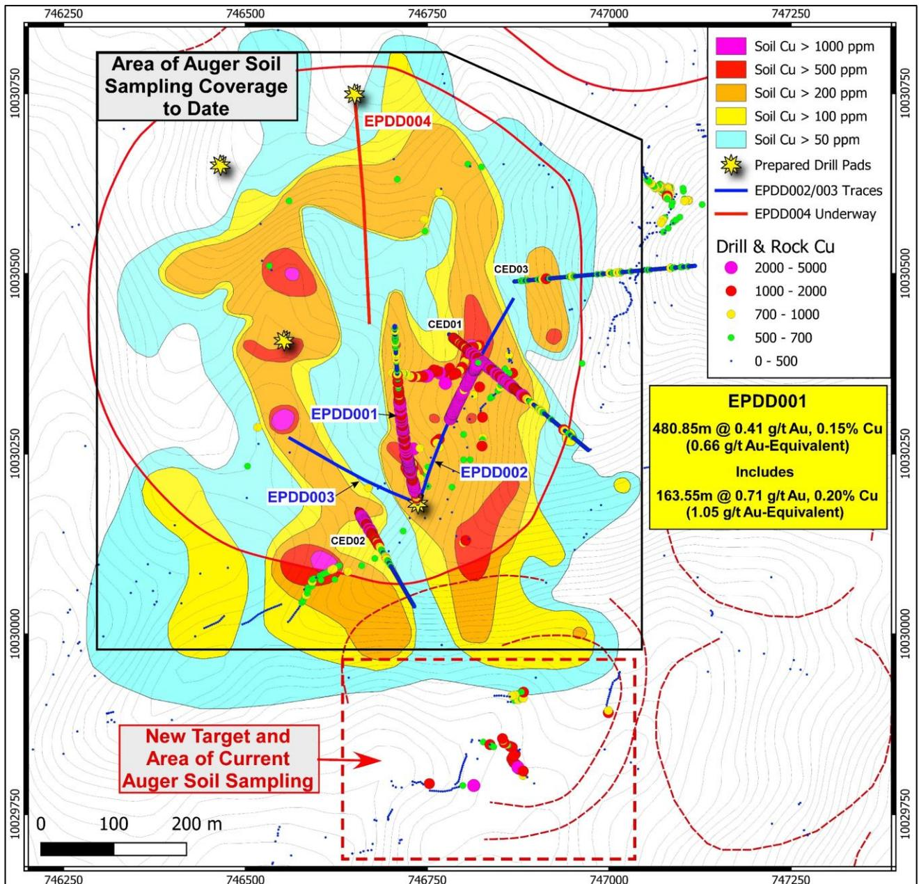
**Figure 4:** Auger soil sampling image showing the coverage area of soil sampling to date and the current area of sampling to the southeast where copper and gold anomalous rock chip results are associated with a magnetic bullseye anomaly. Note – only the middle portion of hole EPDD002 has been assayed – full assays are expected in early November. CED prefixed drill holes are historical (2012) drilling by Codelco.
