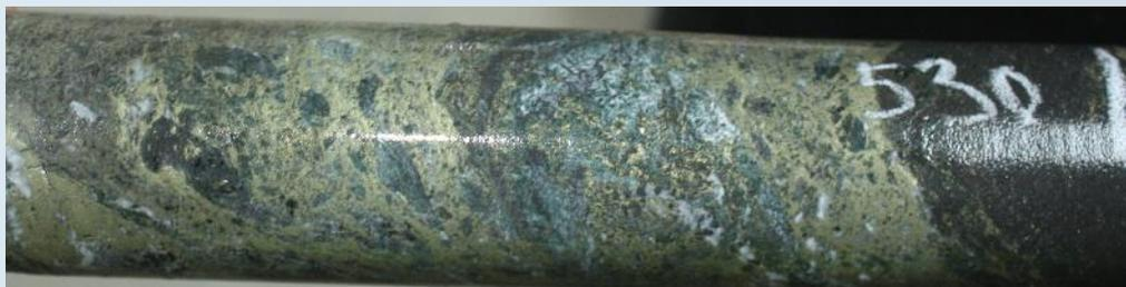
VDD 186; 530m down hole; chalcopryite in altered basalt
