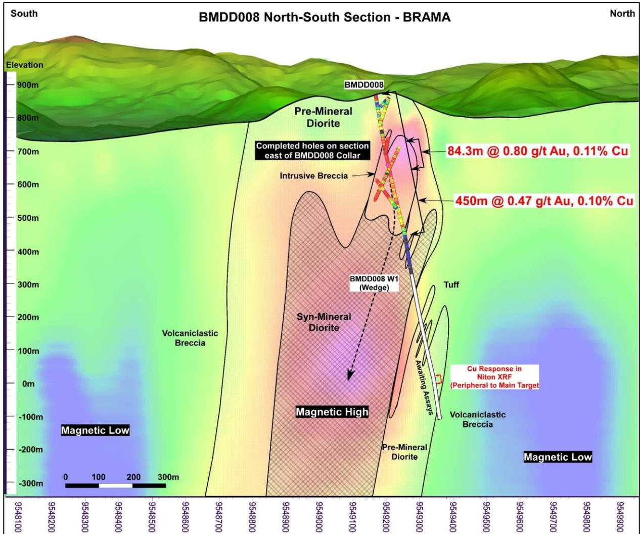
Figure 1: Brama cross section showing a slice through the new 3-D magnetic model with drill hole BMDD008 and new wedge hole BMDD008W1.
