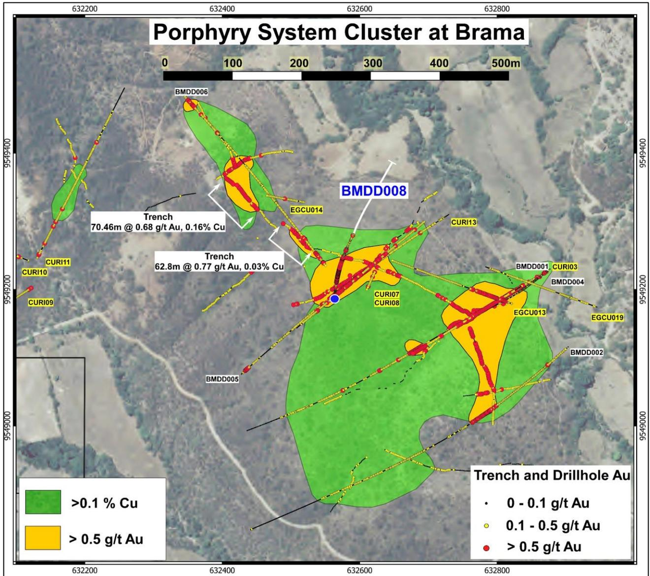
Figure 2: Brama gold-copper porphyry plan view showing higher grade gold domains within a broad lower grade copper halo covering 700m x 500m.
