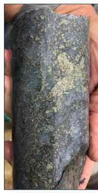
LMDD002, 890.5m, coarse grained chalcopyrite + pyrite
