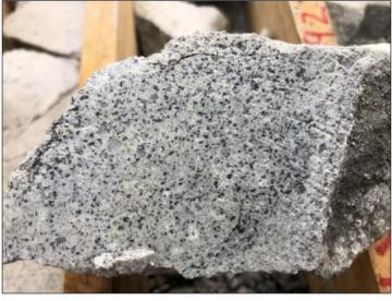
LMDD004 at 68.18m showing black chalcocite and bornite (copper sulphide species) spots through vuggy silica and clay altered volcanic rocks in a 'high sulphidation system. The interval 68 – 69.6m returned assays of 1.11% copper, 0.2g/t gold, and 5.4g/t silver.
